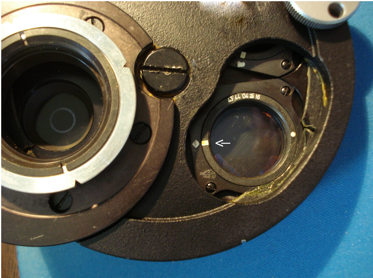
Underside of condenser 46 52 85-9901 with cover removed, showing the condenser prism 43 44 94 for objectives 16x and lower. Arrow indicates the setting for T : square mark opposite white index. (Photo by author).
