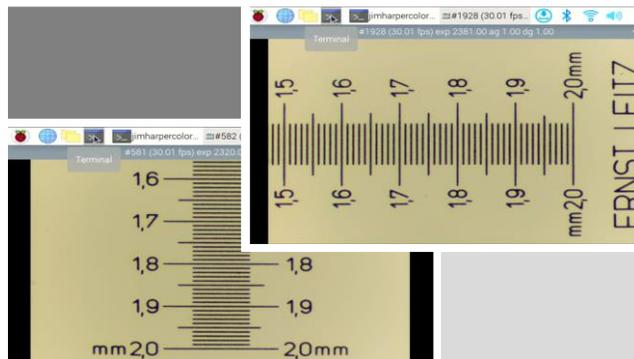
The calibration process uses an image of a scale calibration slide in both horizontal and vertical directions. The camera magnification factor for the Pi Camera is significantly different in the x and y directions. Fortunately, calibrating the ImageJ software automatically adjusts for the camera magnification factor once it is calibrated for a particular objective / projection lens and camera position on the microscope.
