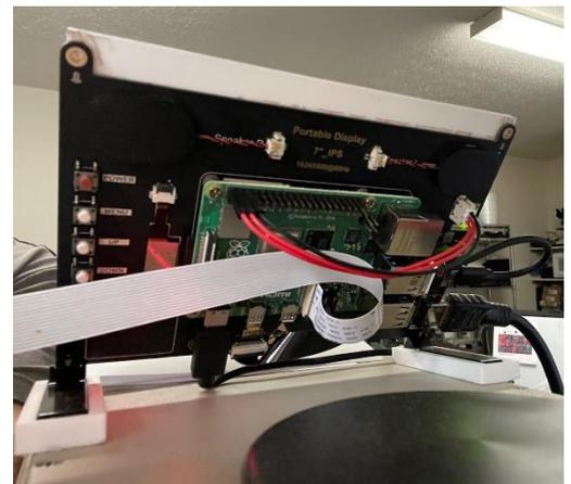
printed cover to project the electronics of the camera. A 1-meter ribbon cable connects the Pi Camera to the computer—long enough to reach the other scopes. 3D Printed adapters to the Leitz and the Wild microscope let me move the Olympus mount from scope to scope.
