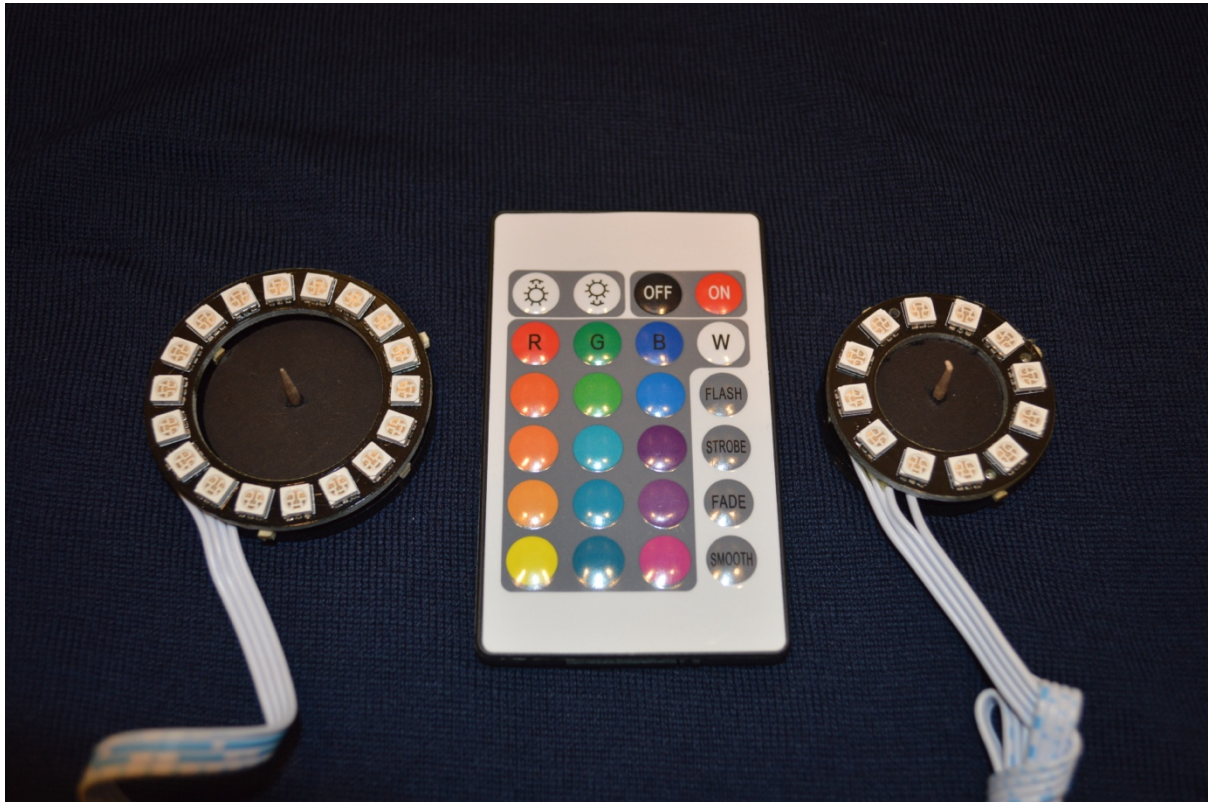
Figure 2. Controllable multi coloured LED rings mounted as per text.
