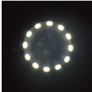
Figure 6. View down phase telescope. If LEDs are positioned further laterally then this will become dark field.
