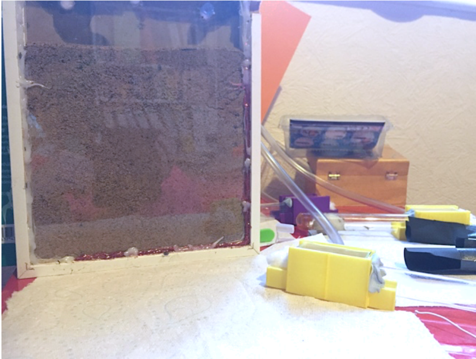
Figure 12: A full Ant Tube, Ant Gateway, and Ant farm setup.
