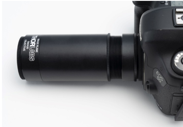
Tube lens mounted and ready to be adjusted so that an object at infinity is in sharp focus.
