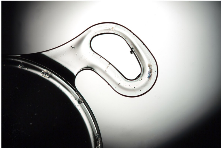
Figure 6. Bausch and Lomb 3D lens haptic detail. Shows scratches on surface due to handling after hardening.
